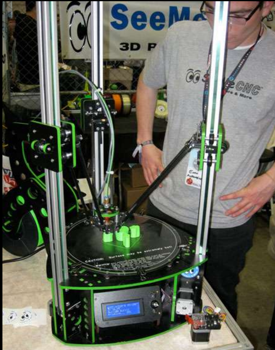
Here's a 3-D printer with non-orthogonal axes. This design always loads the actuators in the same direction, eliminating backlash.
