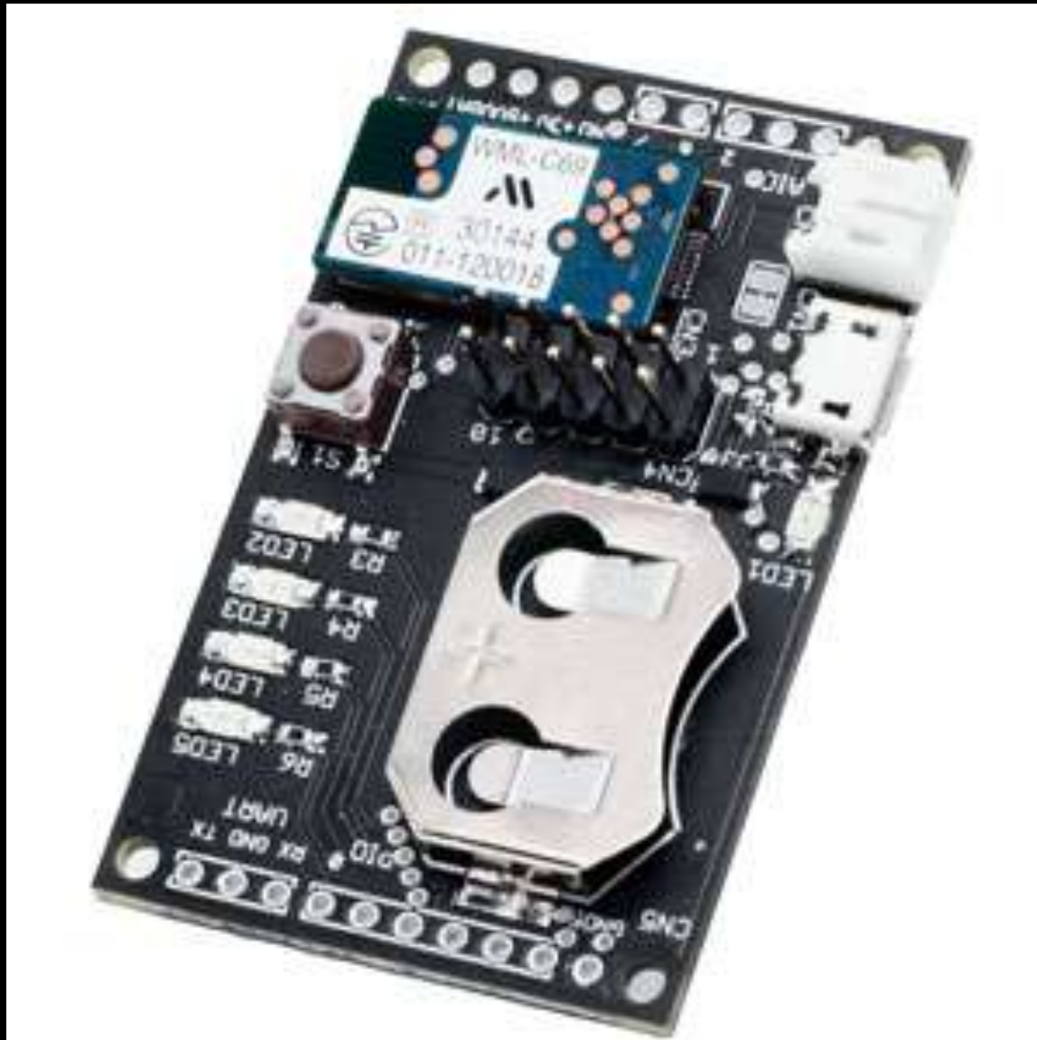
Konashi, a programmable physical computing toolkit that allows developers to wirelessly expand the I/O of a smartphone or tablet.
