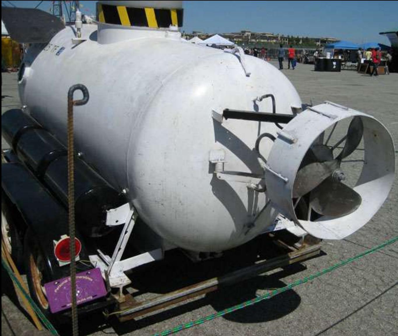
The sub has buoyancy tanks (black near the bottom), a hydraulic motor thruster, and pitch planes. It's done about 25 dives to date.
